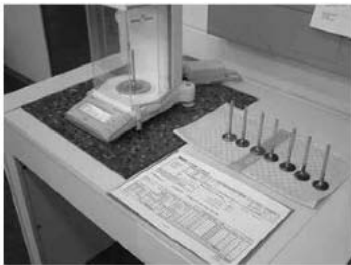
Figure 9. Deposit mass determination of IVD
