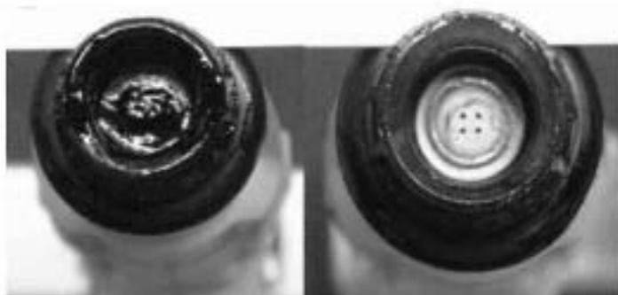
Figure 10. Visual rating of injectors. Dirty Injector (left) and Clean Injector (right)
