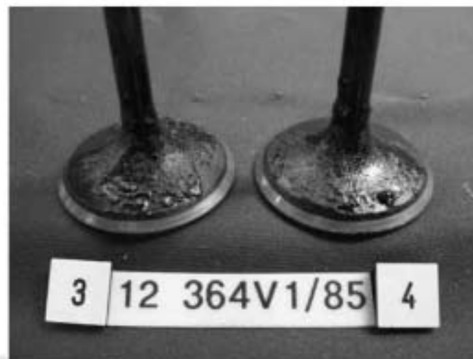
Figure 11. IVD after 60 hours with unadditized E85
