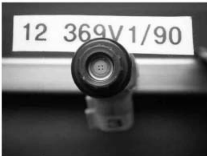
Figure 14. Injector appearance after 60 hours with unadditized E0
