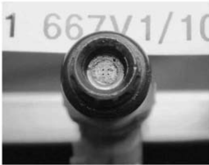
Figure 17. Injector deposits after 60 hours with unadditized E85 / without EGR and blow-by
