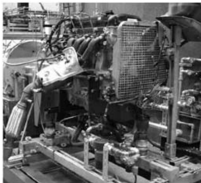
Figure 6. Test engine (FORD 1.8-l-Duratec Flexi Fuel) on test bench
