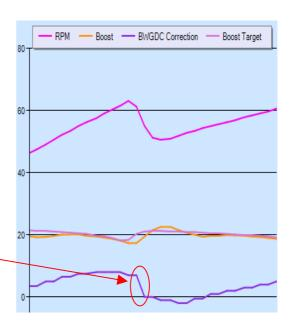
Note 1: This patch checks RPM and error-correction factor at each boost EC interval.
