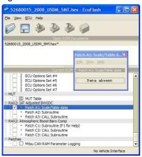
2. Under the window's topbar menu *Edit* heading, choose *Increment*. The item's displayed *patch* state should change, eg.
