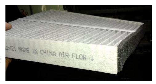
Place the filter in the area you cut out. There are two notches on the bottom to align the filter
