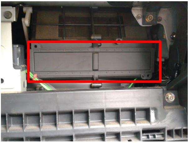
Cut the plastic out with a utility blade to allow access into the filter location
