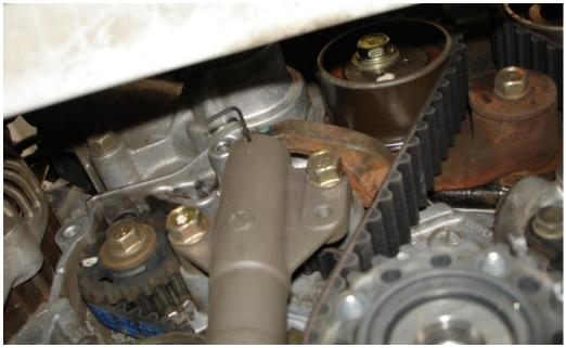
17- Install the Crankshaft Bolt and tighten the 22mm bolt to 123 ft-lb.
