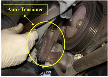
5- Remove the Water Pump Pulley, Qty4 10mm bolts.
