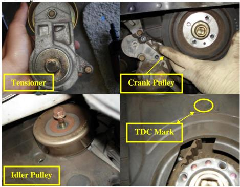
9- Before we remove the Timing Belt Lower Cover, we need to align the Camshaft Sprockets (cam gears), and the Crankshaft Sprocket to TDC. Using the Breaker Bar, turn the Crankshaft Sprocket Clockwise until the Camshaft Sprockets and Crankshaft Sprocket align with TDC. Note the Timing Marks (notches) on the Valve Cover. The Crankshaft Sprocket should also align with the "T" on the Timing Belt Lower Cover. Finally, we can remove the
