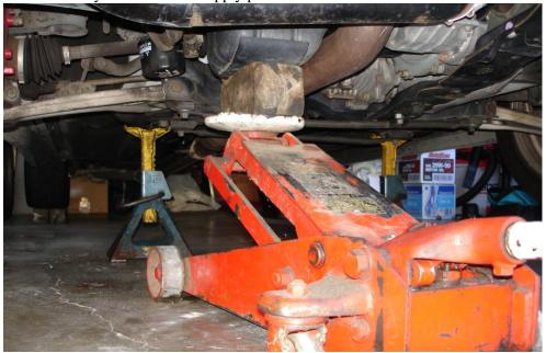
3- Relocate your Power Steering Reservoir Tank, Qty2 12mm, to the side in order to make room for your working area. Next remove the engine mount, Qty3 14mm nuts on engine side and 19mm socket with 17mm open end wrench on the backside. Remove complete mount with rubber inserts.
