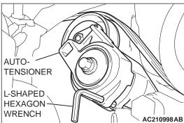
Securely insert the spindle handle or ratchet handle with a 12.7mm (1/2-inch) insertion angle into the jig hole of the auto-tensioner, and turn the auto-tensioner counterclockwise until it hits the stopper.
