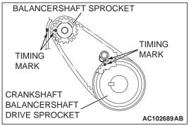
Turn the crankshaft clockwise two turns to set number 1 cylinder to TDC of its compression stroke and check that the sprocket timing marks are aligned.
