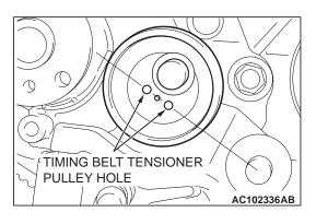
>>E<< TIMING BELT TENSIONER PULLEY INSTALLATION Temporarily tighten the timing belt tensioner pulley as shown.
