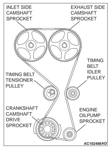
(1) Pass the valve timing belt around the crankshaft camshaft drive sprocket, the engine oil pump sprocket and the timing belt idler pulley in that order.
