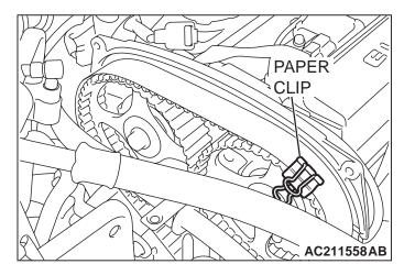
(2) Pass the valve timing belt around the exhaust-side camshaft sprocket, and hold the valve timing belt with paper clips.
