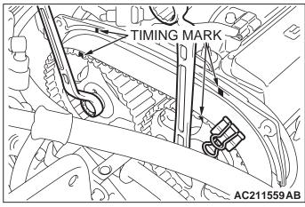
(3) Use two wrenches to align the timing mark on the rocker cover with that on the camshaft sprocket. Pass the valve timing belt around the inlet-side camshaft sprocket.
