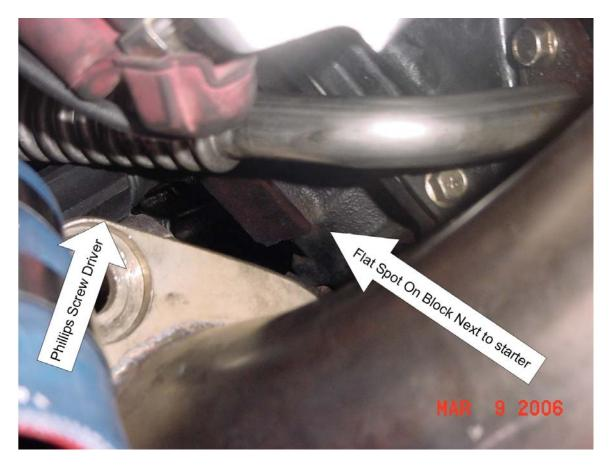
**Step12**: now you're ready to remove the timing belt, with all of your marks on TDC, loosen the 12mm bolt 11A-50, #7 which should unload the tension off the timing belt. You can rotate the pulley counter-clockwise to create more slack if needed. Now remove the timing belt.
