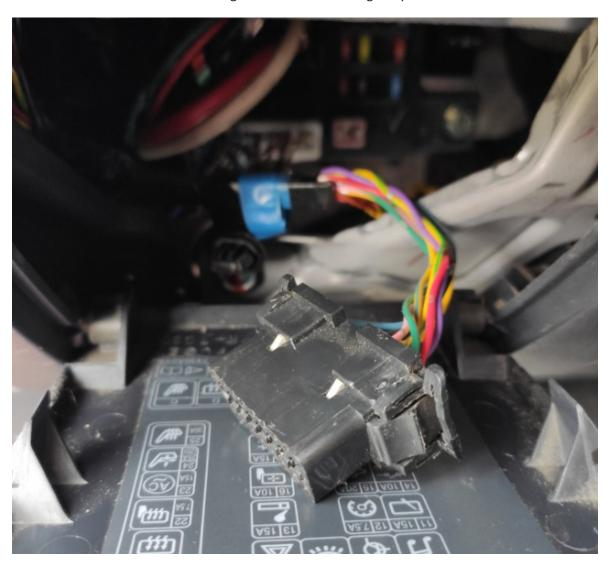
Now we have to remove the little gray tabs that hold the terminals in place. This is achieved by pressing on the little tabs on the front- and backside of the connector respectively.
