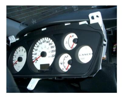
Now that the gauges are exposed, gently pry out the needles, remove the gauges, and replace the two bulbs shown. I didn't finish this part, because I left mine the stock color.
