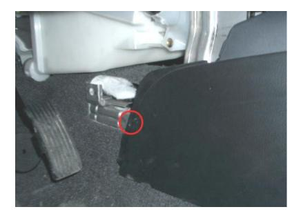
Now to the right passenger side. This panel is completely smooth, held in with clips. Pry gently outward with constant force, it should pop right out.
