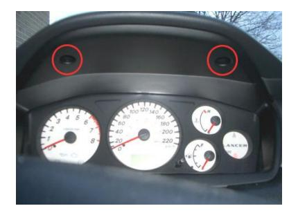
Next, remove the 3 screws holding the gauge cluster in place.
