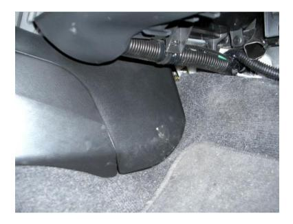
Once again, with the ingenious grommet, push your screwdriver head into the middle, and pop the piece out. You have now completely released the center console, and it should lift right out with the proper angles. If you drive auto, it helps to have your car in neutral at this point to help guide the console out.
