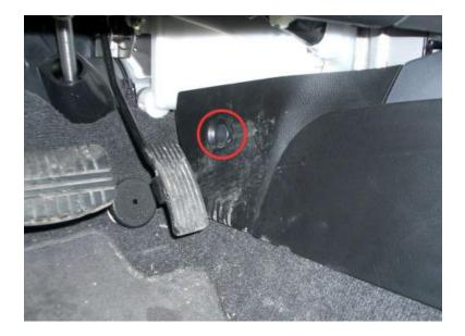
Using the head of your screwdriver, push the center part of this little ingenious device in, and pull out the grommet.
