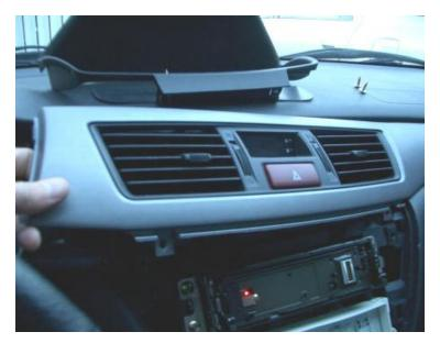
It's a little scary to look at, but here's what you end up with. Disconnect the two cables for the clock and hazard lights.
