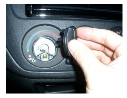
Unscrew these two screws holding the knob controls to the face plate.
