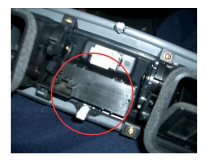
Now you have access to the clock piece. Four tabs, two at the top and two at the bottom hold the clock in. Gently undo these to release the LCD.
