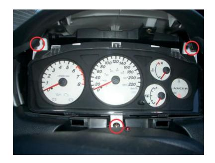
With the gauge cluster loose, pull it slightly out of its sitting place. Now on to the climate controls. Twist all knobs all the way to the left, this makes it easier to put them back in later. Simply pull them out.
