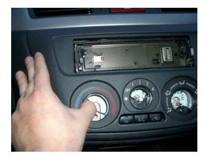
Unscrew these 4 screws, holding in the light guide and the Defogger/AC/Recirc buttons.
