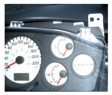
So you want to take this one step further? Undo the clear part of the gauge cluster. There are two clips holding it in at the top, gently push down to release the face.
