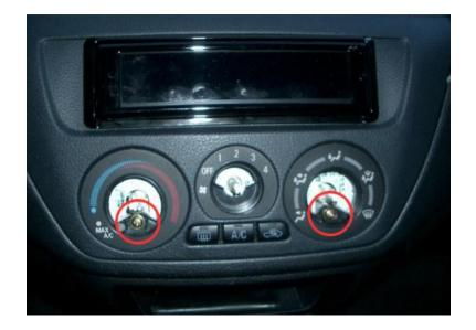
With your fingers in the holes, pull out with even pressure to remove the face plate.
