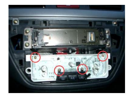
Removing the light guide and buttons should give you clear access to the two bulbs you need to change.
