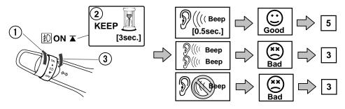
\*) If the buzzer either does not beep or beeps twice, it means that the setting is not effective. Turn off the fog lamps and retry Step 3.
